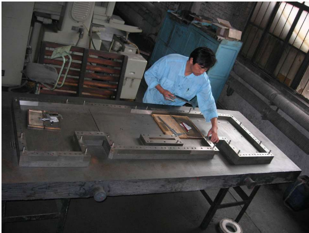
Die ready for stamping of laminations
