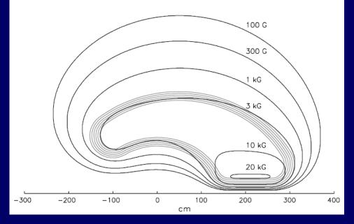
The resulting field is in the  $\phi$ -direction, i.e. always transverse to the particle momentum
