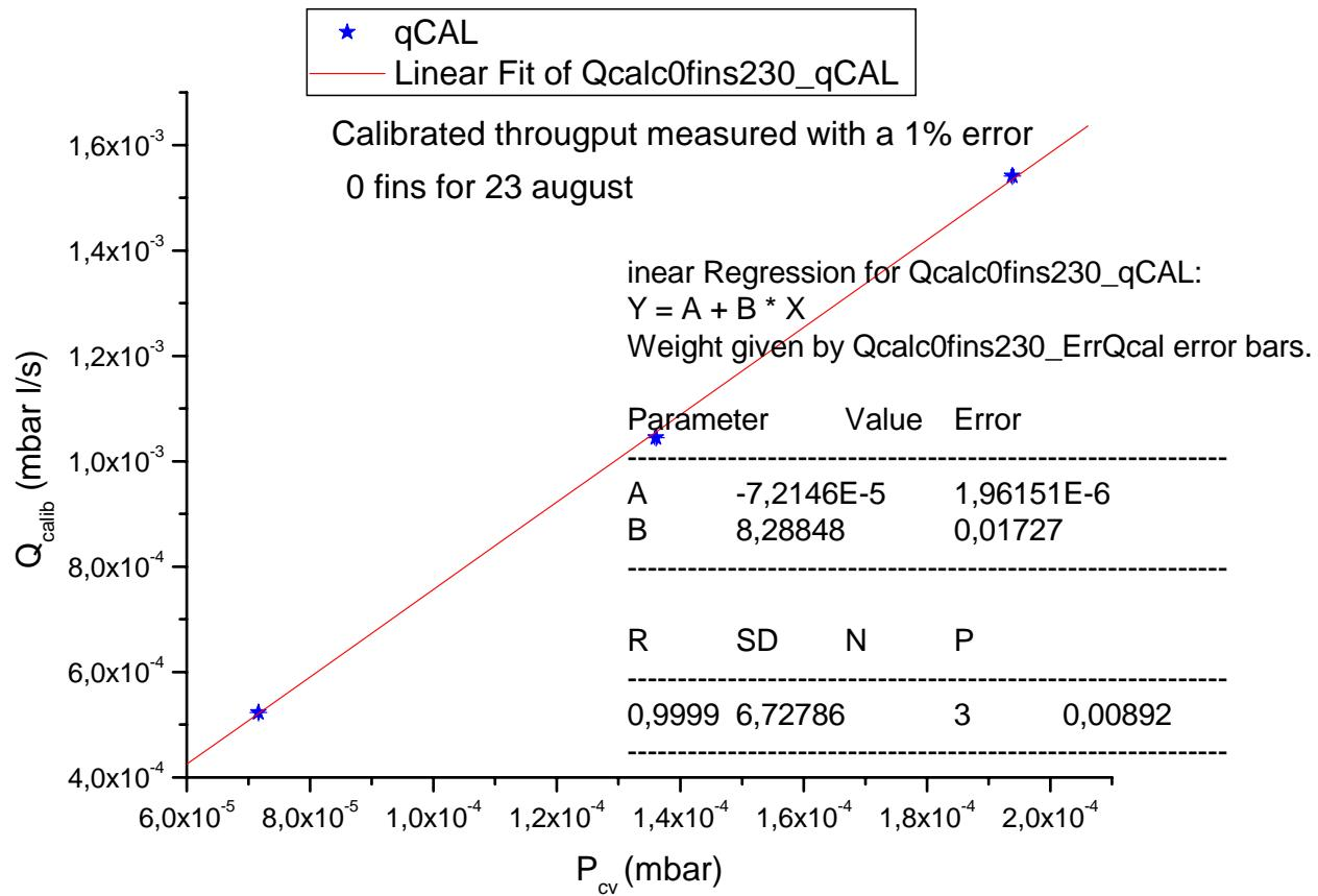
*Q calibration curve derived for all finned tubes*
