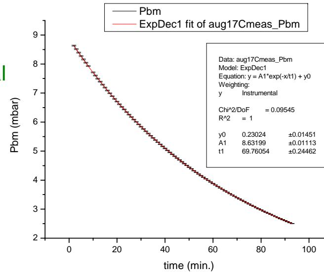
$$C_{cal} = \frac{V_{cal}}{\tau}; \text{ inoltre } \frac{\delta C_{cal}}{C_{cal}} = \frac{\delta V_{cal}}{V_{cal}} + \frac{\delta \tau}{\tau}.$$
