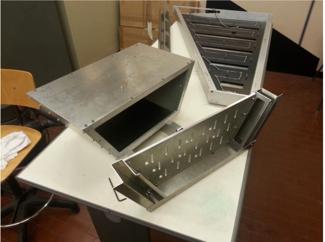
Figure 12: Assembling of the electronic panel and cooling prototypes.
